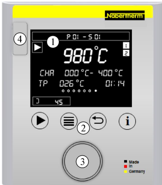
Fig. 25: Control field B400/C440/P470 (similar to picture)
